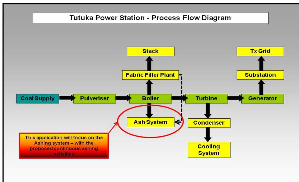
**Figure 4.1:** An overview of the activities on site and where this project fits within the power generation process
