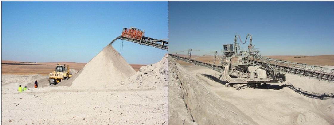
**Figure 4.4:** Stacker being used to dispose of ash at the Tutuka Power Station
